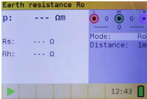
Figure 5.50: Specific Earth Resistance (Ro) measurement menu
