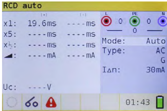
Figure 5.20: Step 4.1 RCD autotest results
