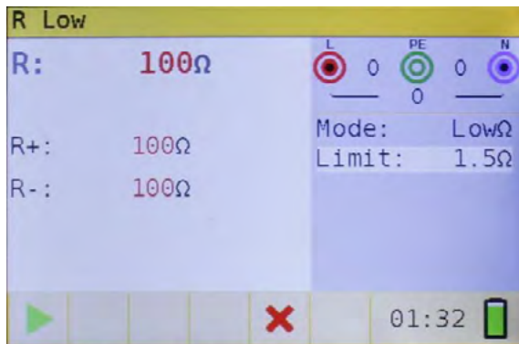
Figure 5.7: Examples of R Low resistance measurement results
