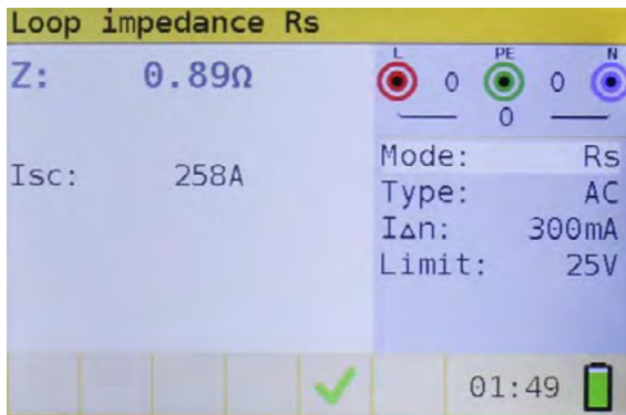
Figure 5.34: Example of fault loop impedance measurement results using Rs function
