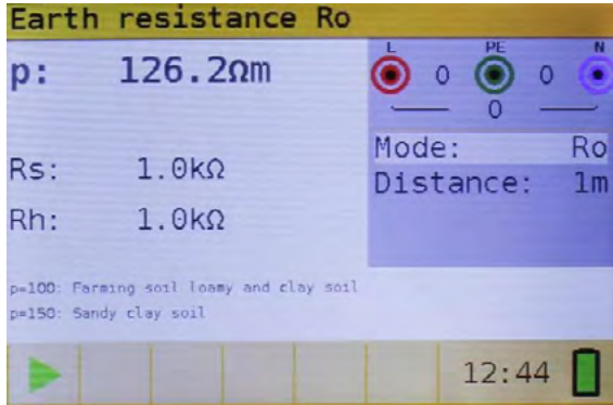
Figure 5.52: Example of specific earth resistance measurement results
