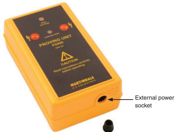
If internal batteries are fitted they will be disconnected by the insertion of the jack plug. If however, the internal batteries are not the intended primary power source, it is advisable to remove them to prevent damage from leaking batteries.
