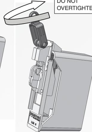
Adjust sliding cover to suit overall length of fuse holder base.
