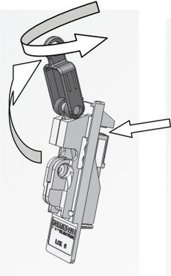
Place jaws centrally over end wall of fuse holder base.
