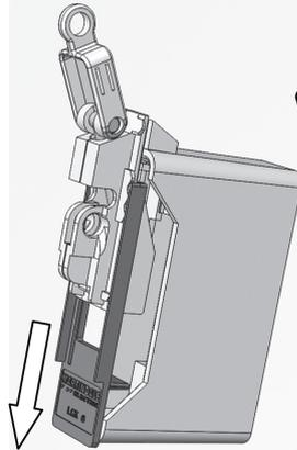
Close toggle. Check that the locking off device is secure.
