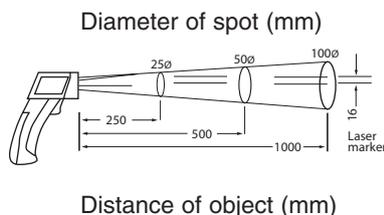
Spot size increases with distance from the probe tip as shown (Spot Diameter measured at 90 % Energy)
