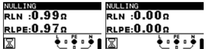
Fig 4. Example screen displays during nulling
