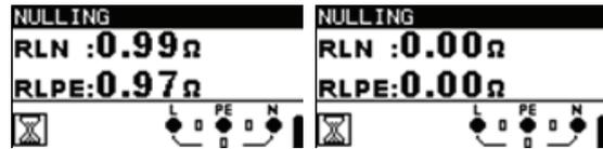
Fig 4 Example screen displays during nulling
